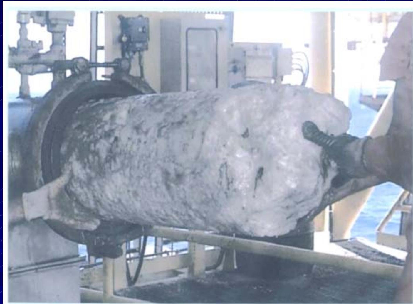
Hydrate Plug coming from the pipeline into a platform
