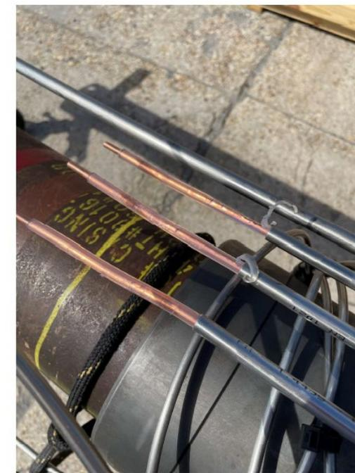
Figure 20. Damage to ESP leads after pulling adapter / hanger
