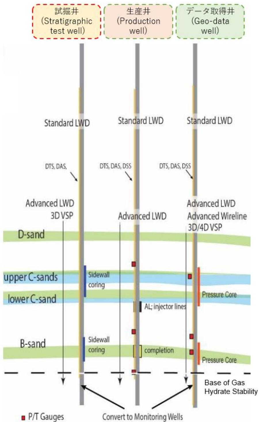
**Fig.2:** Assumed wells and the monitoring equipment arrangements
