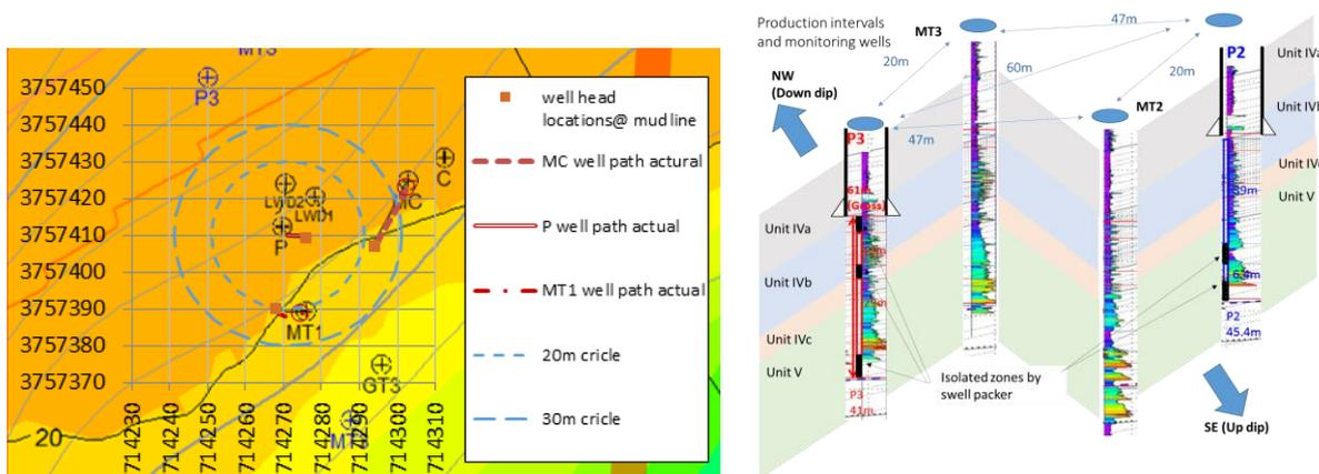
Fig. 1 Borehole configuration of first (left) and second (right) offshore production tests. In first test, some well inclination was observed, and projected well trajectories were drawn using red lines. As a result, production well was drilled in downdip direction. For second test, monitoring and producer boreholes were intentionally drilled at vertex points of a parallelogram to distinguish MH dissociation-induced temperature drop and influx of cool fluid.
