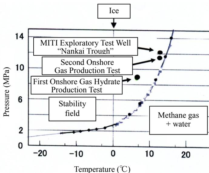
Figure 2-1 Stability field of methane hydrate
