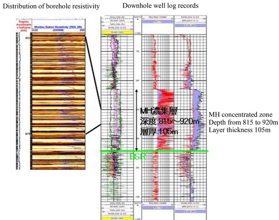
Figure 5-2 Example of the downhole well log data denoting turbidite sand and mud alteration layers
