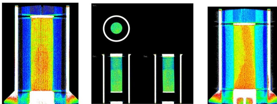
Figure 8-2 High speed X-ray CT visualized images indicating the dissociation processes of various decomposition methods
