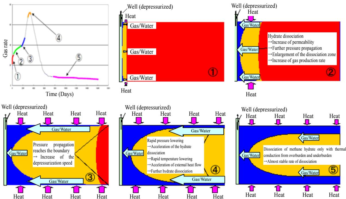
Figure 7-5 Behavior of gas production by the depressurization method accompanied with the heat supply from the adjacent formations and the change of the methane hydrate dissociation zone
