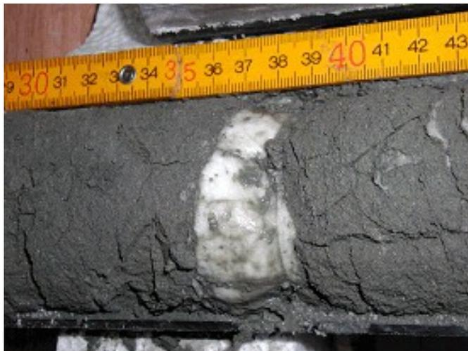
Figure 2-4 A massive sample of methane hydrate in muddy sediment
