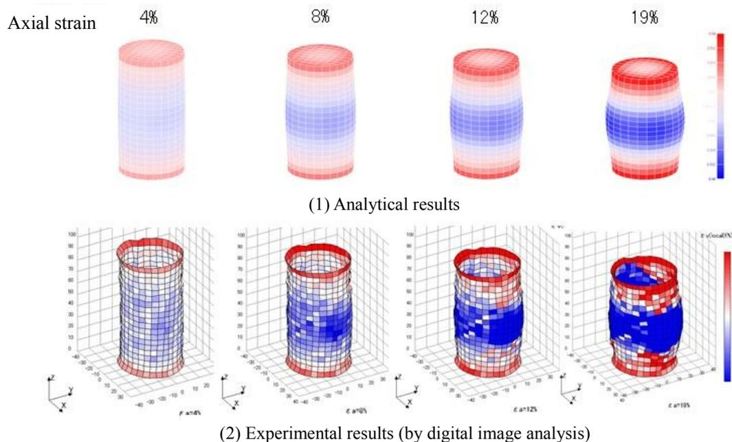
Figure 5-6 A result of the numerical analyses for the tri-axial compression tests of the core samples obtained from the METI/MITI Exploratory Test Wells (the distribution of volumetric strain)
