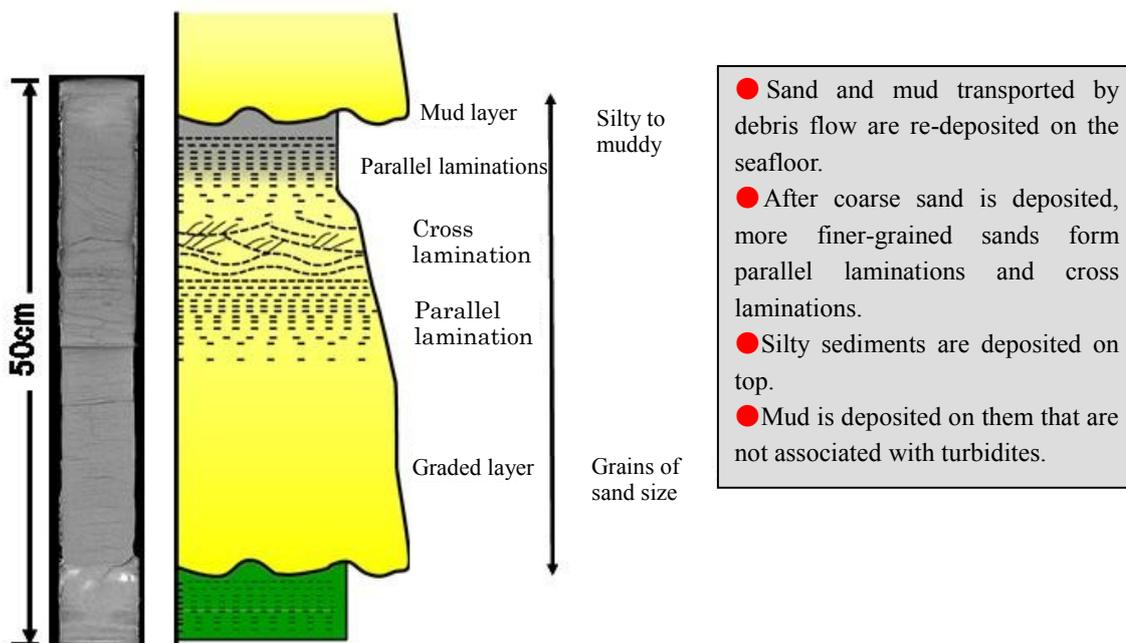
Figure5-3 Geological characteristics of turbidite sand and mud alternation layers
