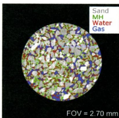
Figure 8-1 Four-component discrete image of the sandy core obtained from the METI Exploratory Test Wells “Tokai-oki to Kumano-nada,” sand, methane hydrate, water, and methane gas
