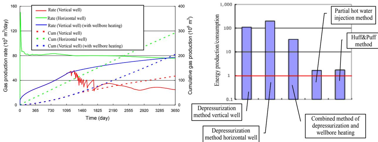
(a) Example of the prediction results of gas production behavior by the depressurization method
