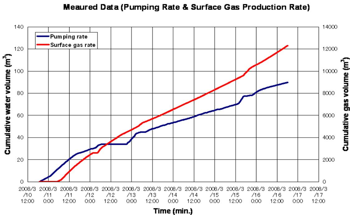
Figure 6-2 Measured production volumes of cumulative waters (blue line) and gases (red line)
