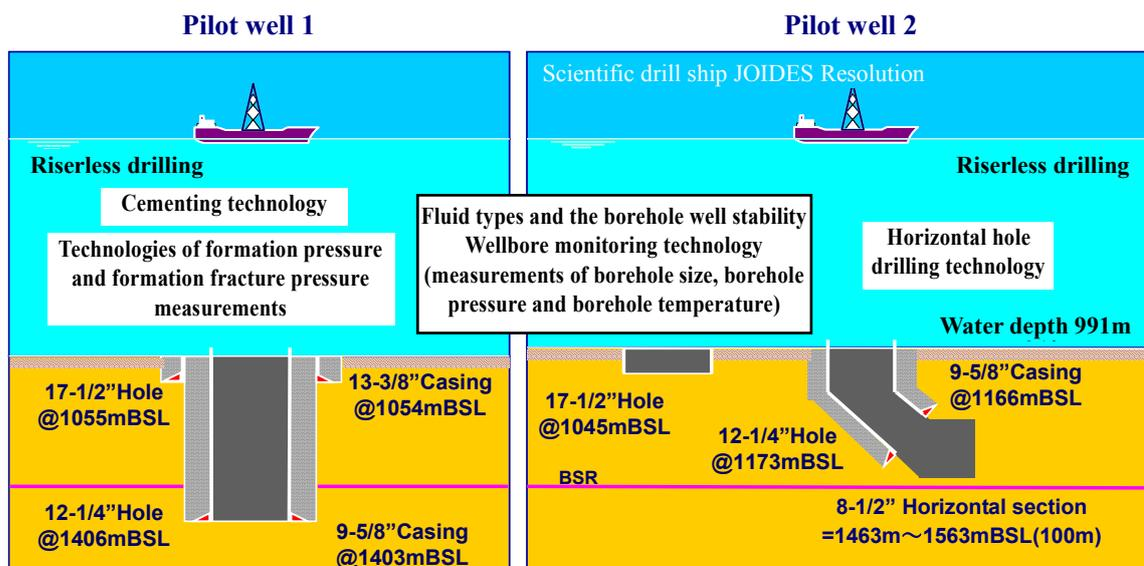
Figure 8-3 Schematic diagrams of the experimental well 1 and 2
