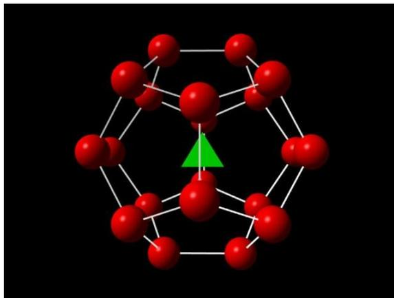
Figure 2-2 A small cage composed of the crystalline structure of methane hydrate
