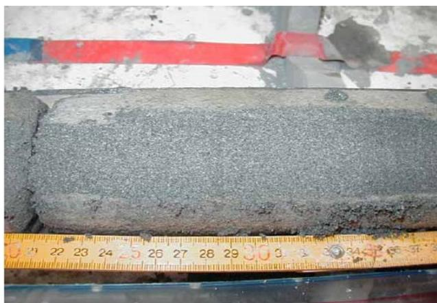
Figure 2-3 A core from the sandy methane hydrate-bearing layer
