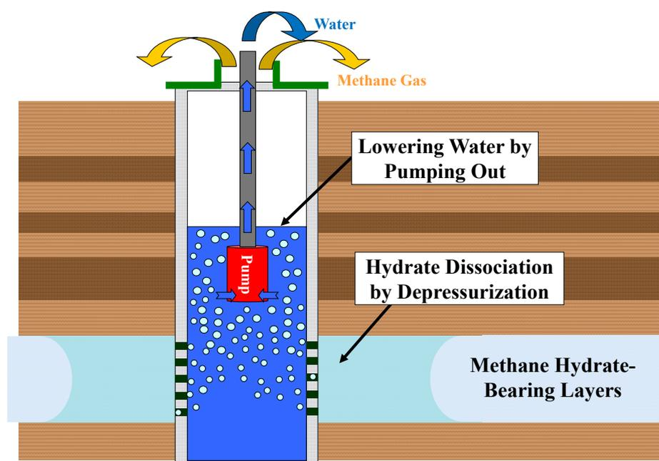
Figure 6-1 Schematic diagram of the depressurization method
