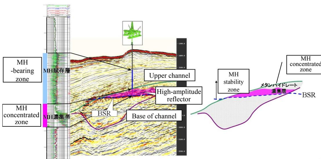
Figure 5-4 Example of methane hydrate concentrated zones
