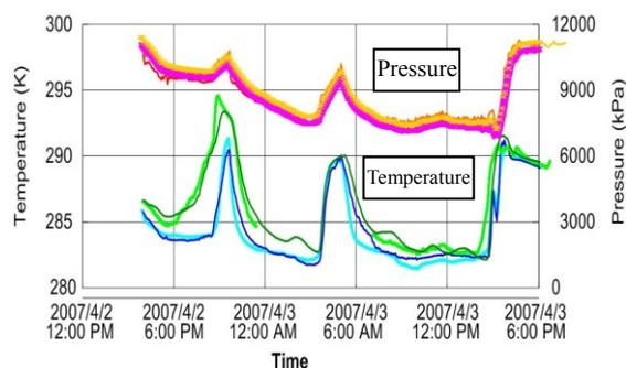
(b) Matching of the borehole temperature and pressure
